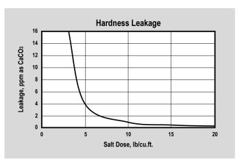
CAPACITY AND LEAKAGE — Capacity and leakage data are based on 2:1 Ca:Mg ratio, 500 ppm TDS as CaCO3, 0.2% hardness in the salt, and 10% brine concentration applied co-currently through the resin over 30 minutes. No engineering downgrade has been applied.
