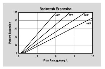
BACKWASH — The graph above shows the expansion characteristics as a function of flow rate at various temperatures.
